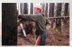
Motor-Manual Logging Operation – A chain saw operator fells the trees, a skidder operator skids them to a staging area, or landing, where a slasher operator, or sometimes a manual chain saw operator, cuts them to length, and a loader operator sorts them and lifts them onto a truck. A truck driver trims the load and transports it to market. On a "high-lead" operation, a suspended cable (rather than a skidder) conveys the harvested log to the landing.
