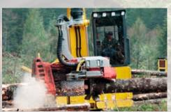
Cut-To-Length Operation – An operator within a cab with computerized measurement capabilities severs the standing tree and, still gripping it with a processor-head, strips off the limbs, and cuts it to specified lengths. A wheeled or tracked forwarder then picks up the processed pieces and transports the load to the landing. A loader then transfers the fully processed logs to the truck for transport.
