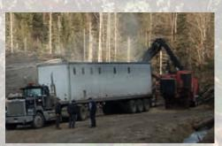
In-Woods Chipping Operation – Many pulpwood and forest biomass loggers today convert their harvest to chips in the woods and deliver chips, rather than roundwood, to mills that use wood in that form. A grapple operator at the landing pushes harvested trees into the in-feed, where a mechanized process chips or grinds the stems and blows the resulting product into a van for transport to the mill.
